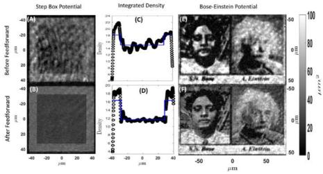
**Figure 1:** Experimental atomic density (A) of initial guess as to the "optimal" DMD pattern to create 2 grey level boxes and (B) after feedforward. (C,D) are the mean integrated atomic density profiles of (A,B). (E,F) are as per (A,B) but for the creation of an atomic density pattern depicting Bose (Left) and Einstein (Right).
